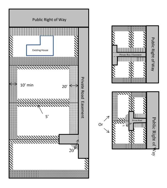
Figure 5-10: Example Private Road Easement Setback Measurements [ADDED 06-07-2018]
