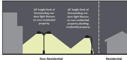
Figure 5-15 **Shielding Provisions for Outdoor Lighting**
