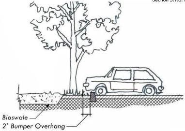
Figure 5-14: Example of Bumper Overhang
